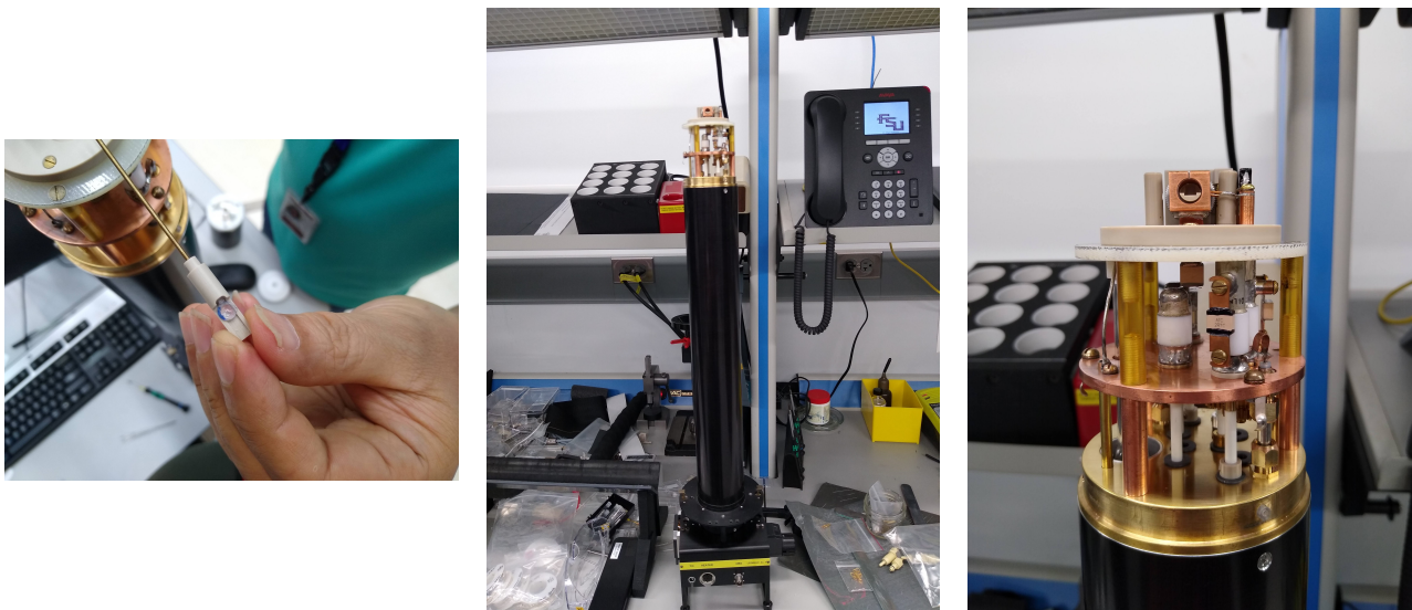
Figure 1: Left: L -NAV crystal on goniometer. The crystal is marked for reference. Center: SCNMR goniometer probe to be used in 14.1 Tesla NMR magnet. Right: Close up view of probe showing its components. On the top is the coil where sample is placed.
