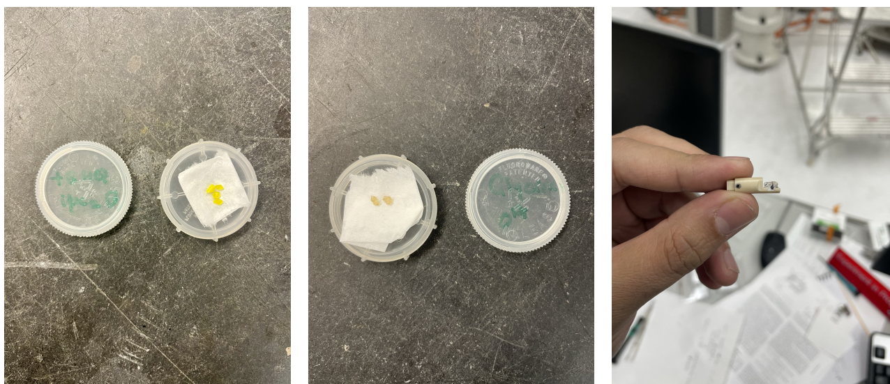
Figure 2: Left: 8-HQ(ipc) _2 B crystals harvested for experiment. Center: Glycine crystals enriched with ^{17}\text{O} . Right: L -alanine crystal on goniometer. The crystal is marked for reference.
